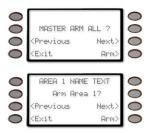
Or press the Next> soft key to view each unarmed area and optionally arm each one. To arm a selected area, press Next> until the desired area appears (Area name text along with Arm Area #?). Then press Arm>.
