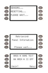
If you enter this function and the detector or sensor resets momentarily, but then returns to a faulted condition, the conditions causing the activation may still be present or the detector may be faulty. Check to be certain that there is no smoke, fire, or other danger present. If you can't reset the detector or sensor contact, your security company.
